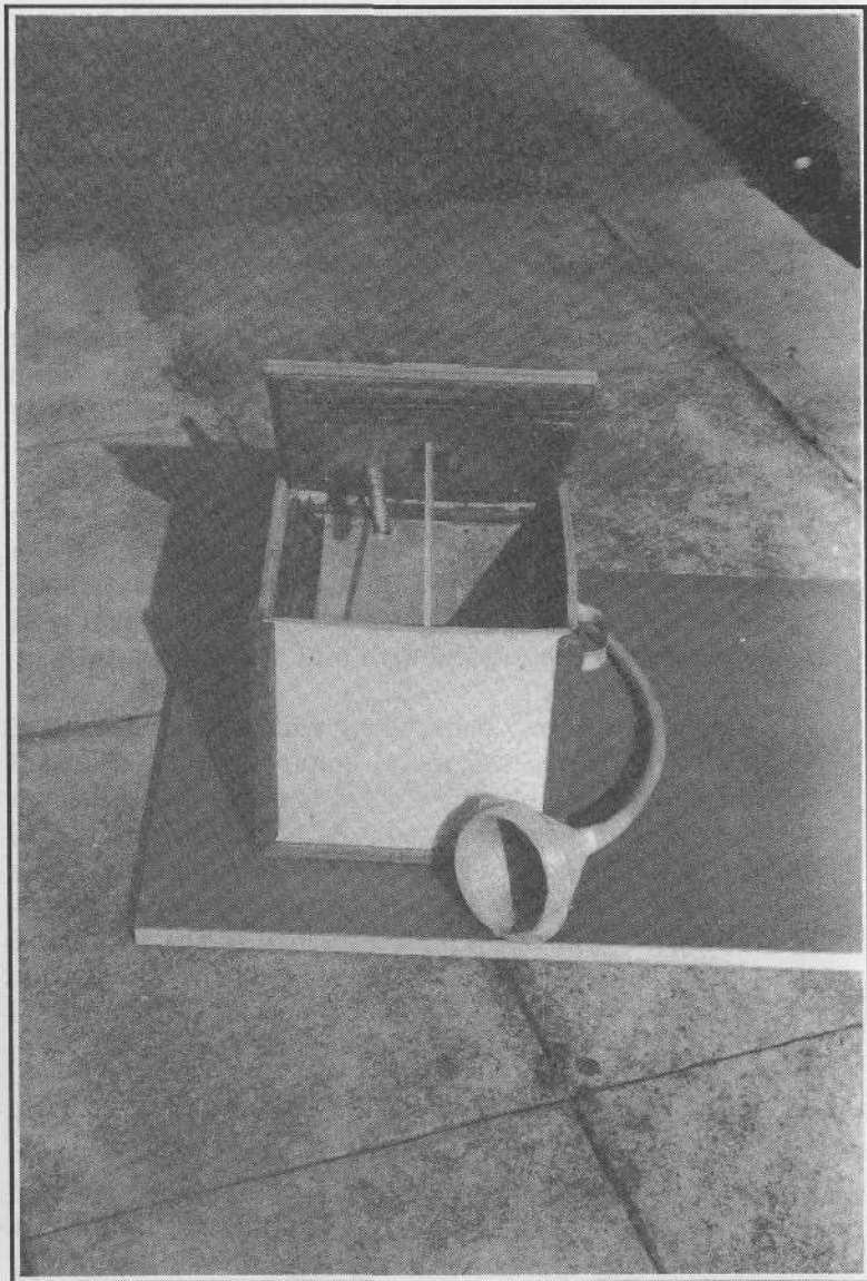
A one-cubic foot, 10-ply accumulator with attached funnel.
