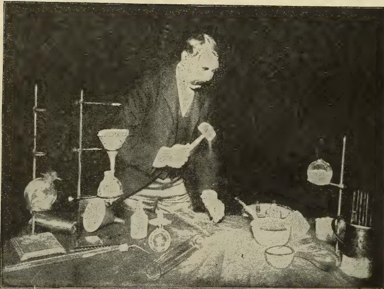
DRIVING A NAIL WITH A HAMMER MADE OF MERCURY FROZEN BY LIQUID AIR.
